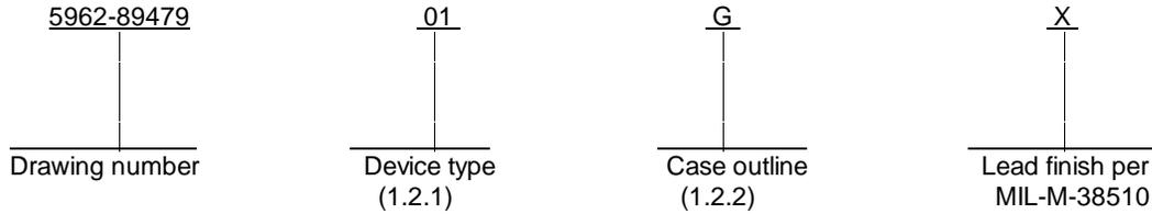
1.2.1 Device types. The device type shall identify the circuit function as follows:
