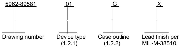
1.2.1 Device type(s). The device type(s) shall identify the circuit function as follows:
