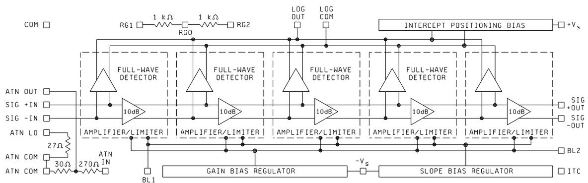
FIGURE 2. Block diagram.
