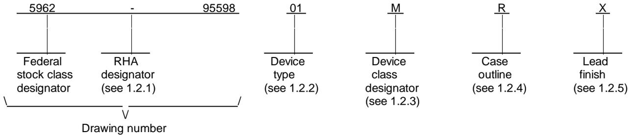
1.2.1 RHA designator. Device class M RHA marked devices shall meet the MIL-I-38535 appendix A specified RHA levels and shall be marked with the appropriate RHA designator. Device classes Q and V RHA marked devices shall meet the MIL-I-38535 specified RHA levels and shall be marked with the appropriate RHA designator. A dash (-) indicates a non-RHA device.
