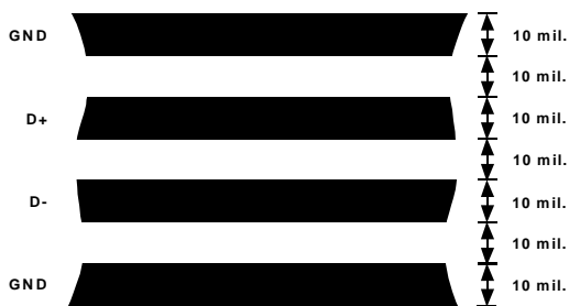
Figure 4. Arrangement of Signal Tracks
