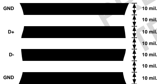
Figure 9. Arrangement of Signal Tracks
