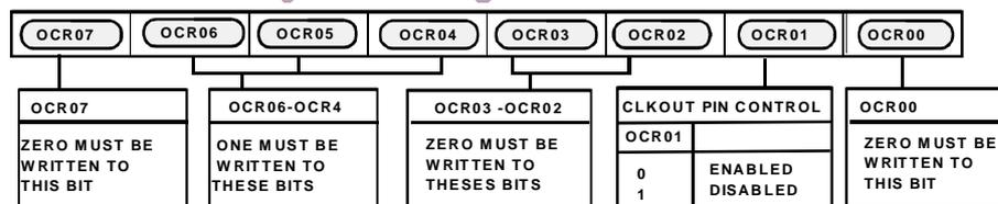
Figure 93. Output Clock Register
