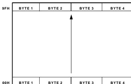
Figure 10. Flash/EE Data Memory Configuration
