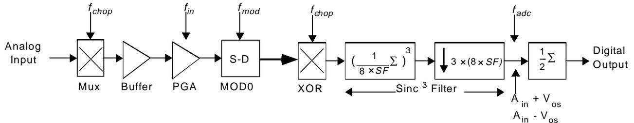
Figure 5. ADuC824 Main ADC Channel Block Diagram
