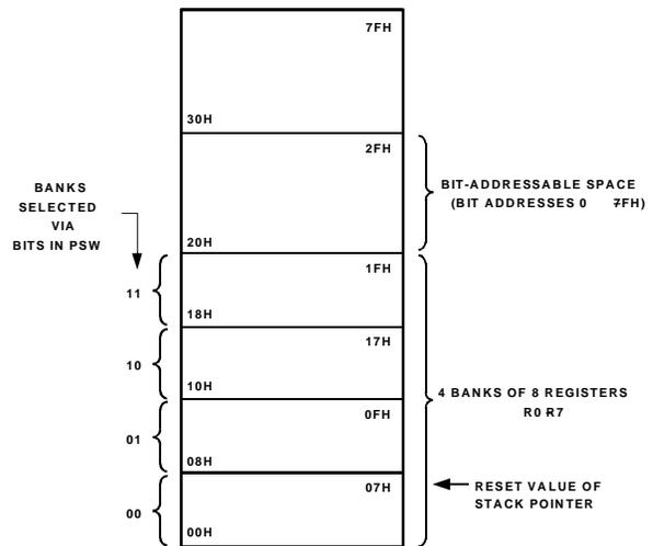
Figure 3. ADuC824 Lower 128 Bytes of Internal Data Memory
