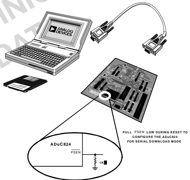
Figure 8. Flash/EE Memory Serial Download Mode Programming
