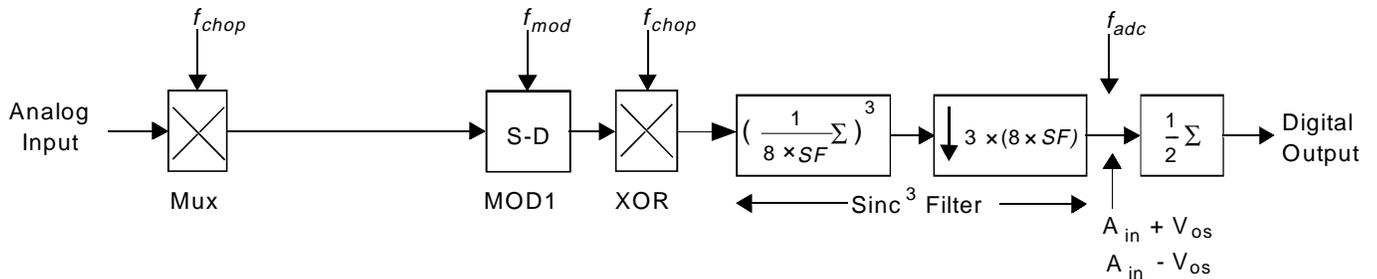
Figure 6. ADuC824 Auxillary ADC Channel Block Diagram
