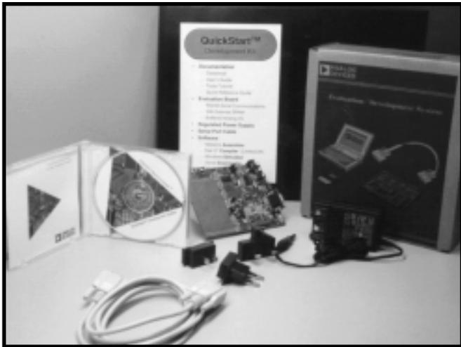
Figure 14. Components of the QuickStart Development System
