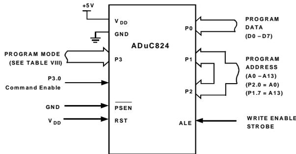
Figure 9. Flash/EE Memory Parallel Programming
