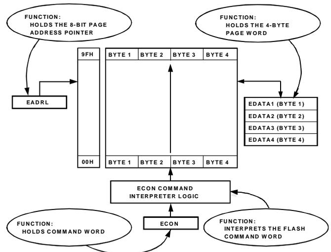
Figure 11. Flash/EE Data Memory Control and Configuration
