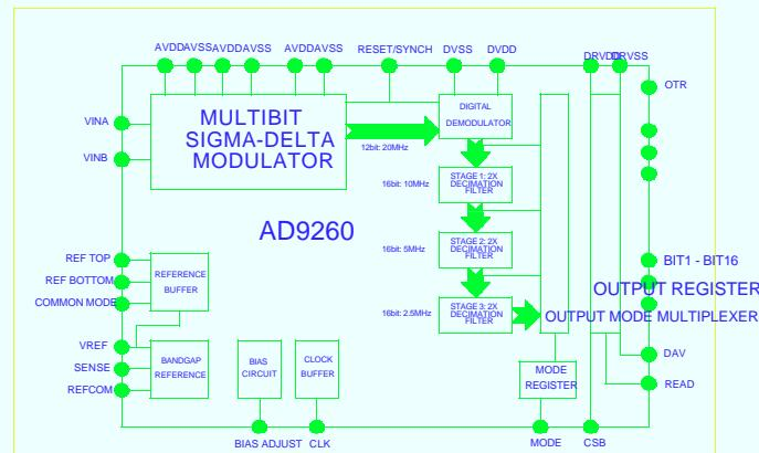
The AD9260 operates on a single +5 V supply, typically consuming 550 mW of power. A power scaling circuit is provided allowing the AD9260 to operate at power consumption levels as low as 150 mW at reduced clock and data rates. The AD9260 is available in a 44-lead MQFP package and is specified to operate over the industrial temperature range.
